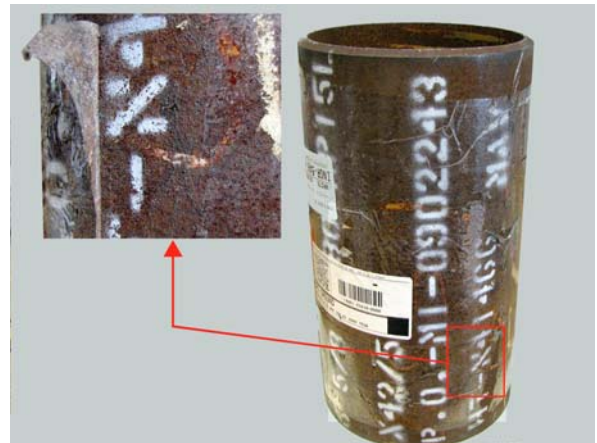
Figure 11: Section of 6 in. diameter API 5L piping used for evaluating corrosion removal performance of bristle blasting tool
